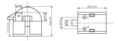
Installation force: 98N Unload force: 25N Flame retardant grade:UL94-V0
