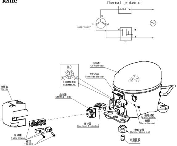
Note: Each of the starting relay, the thermal protector, the terminal cover and the screw assembly is separately provided by our company.
